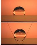
2.0% polymer on glass Water contact angle: 113.3°
