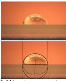
2.0% polymer on glass Oil contact angle: 82.0°
