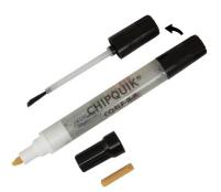
**Specifications** Flux Type: No-Clean Liquid Flux (for Leaded and Lead-Free applications) Flux Classification: ORL0 **VOC Free** VOC Content: Acid Number: 38.0 Total Solids: 4.0% Specific Gravity: 1.01 Packaging: Refillable Pen 6ml (0.2oz) - Two Ends: Tip and Brush Shelf Life: Refrigerated >24 months, Unrefrigerated >24 months
