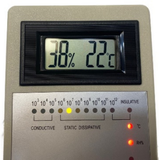
Image 1: Resistance on an ESD work mat (static dissipative)
